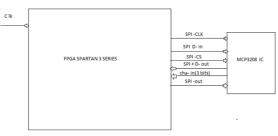
Fig 6: Block diagram of ADC in hardware implementation.
