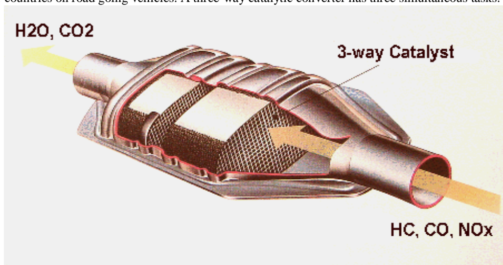
Fig.4.4. Cut Section of Three Way Catalytic Converter
