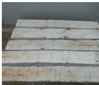
Fig 4.3 failure of beams
