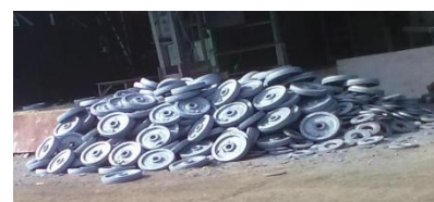
Fig: 7 Blank cutting, saw m/c and Finished gears after forging sequences in forging plant
