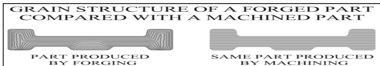
Fig: 4 Grain structure in forging
