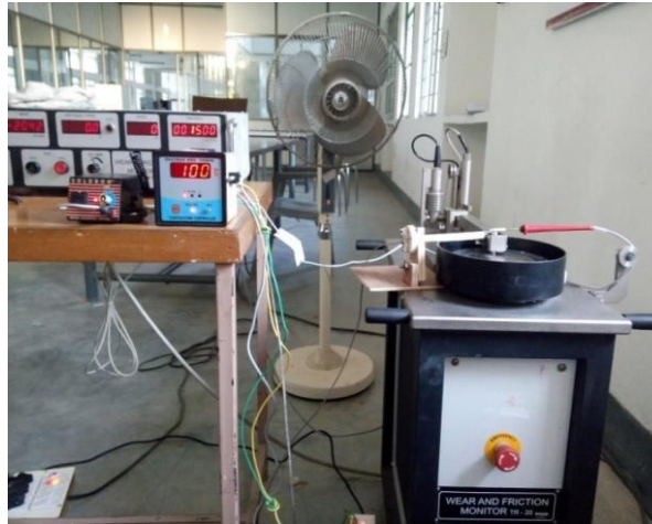
Fig.2 A photograph view of the pin -on-disk type wear testing machine
