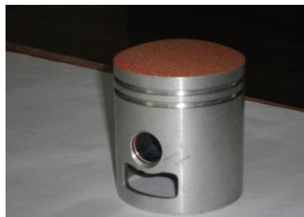
Plate.1. Photographic view of copper coated piston
