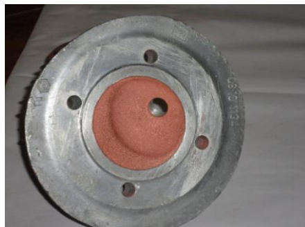
Plate.1. Photographic view of copper coated cylinder head
