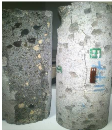
Fig. 3 Failure pattern of vesicular basalt under uniaxial compression
