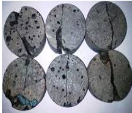
Fig. 5 Failure pattern of vesicular basalts in Brazilian test
