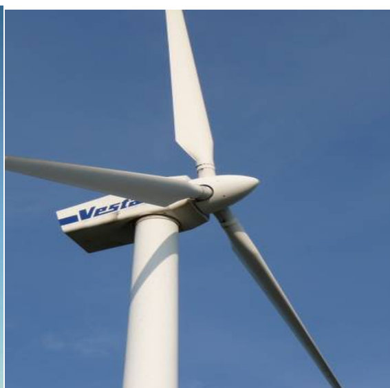
Figure 3.2: Horizontal Axis Wind Turbine
