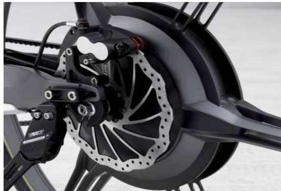
Figure 6: Illustration of Wheel Hub Motor
