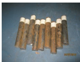
Figure 1. Samples of 41Cr4 Alloy Steel Bars
