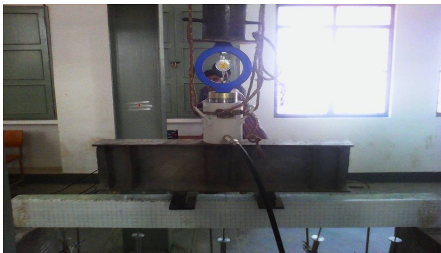
Fig.1 loading arrangement of beam
