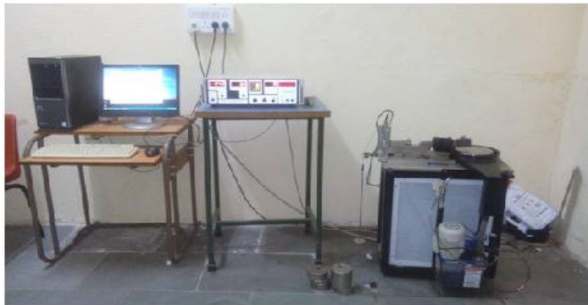
Fig 1: DUCOM friction and wear monitor with pin on disc wear machine.
