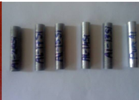
Fig-5. Specimen used for wear test
