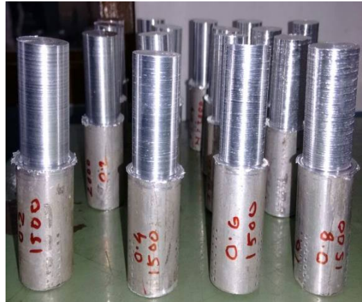
Fig. 2: Aluminium workpieces after turning operation
