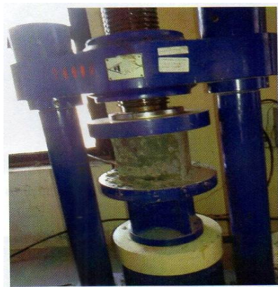
Fig No. 3 Compression Testing Machine. (CTM) Fig.No 4 Precipitation on Surface of Concrete Cube. Figure 3 the cubes ware tested in 2000kn capacity compressive testing machine. Loaded at constant rate of constant rate of loading at 200 kg/cm 2 /min. as per IS : 516-1959 (1999).
