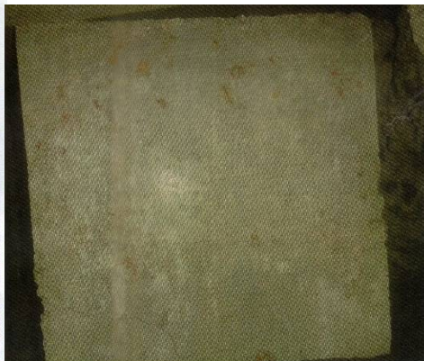
Fig No. 3 Compression Testing Machine. (CTM) Fig.No 4 Precipitation on Surface of Concrete Cube. Figure 3 the cubes ware tested in 2000kn capacity compressive testing machine. Loaded at constant rate of constant rate of loading at 200 kg/cm 2 /min. as per IS : 516-1959 (1999).
