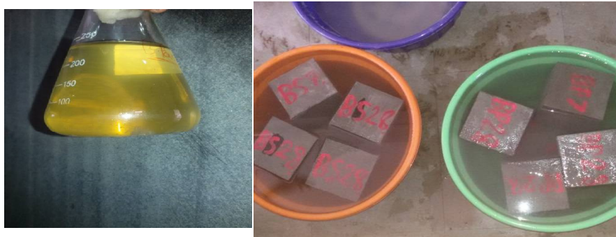
Fig No. 1 Nutrient broth solution Fig No. 2 immersion of Sample in Precipitation of Media
