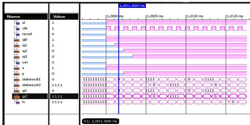
Fig.4.Simulation Result of 4-QAM Modulator
