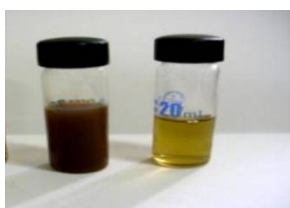
Fig. 5 Photo showing the formation of silver nano particles in yellowish brown colour and the neem flower extract in yellow colour
