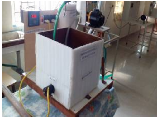
Figure 3 Actual test rig for testing energy storage unit
