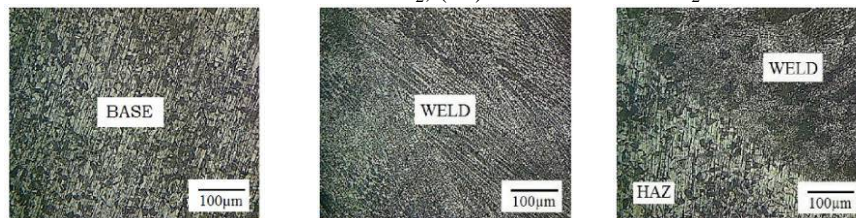
Figure 4. Microstructure of penetration profiles welded under shielding of 100% Ar (P1).
