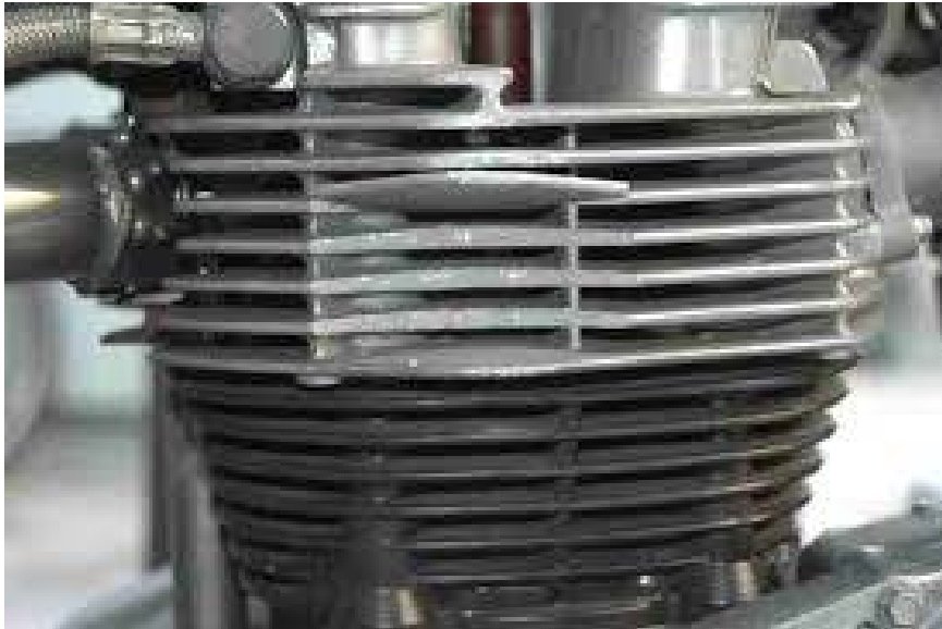
Fig 1.2 Fins in Bike Engine
