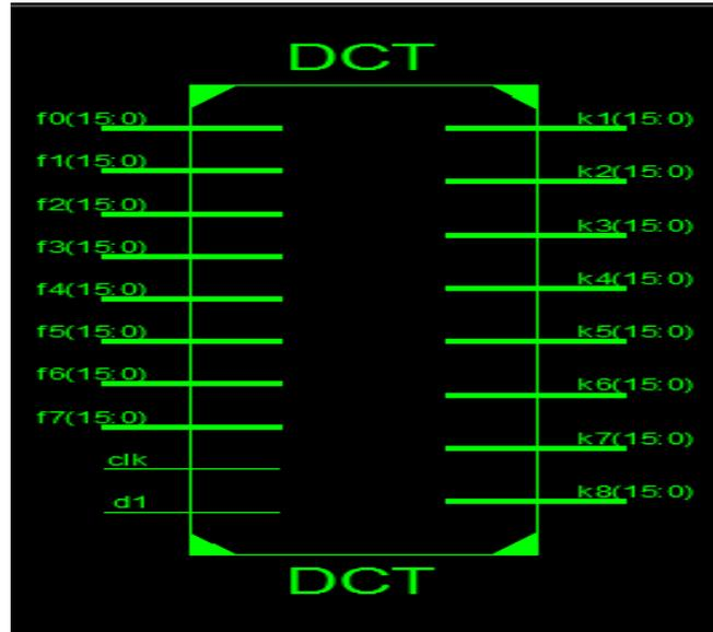
Figure 4: Register transfer Level (RTL) View of 8-point DCT
