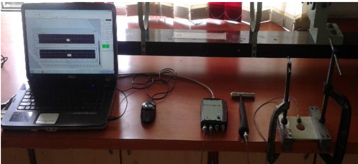
Fig. 4: Experimental setup of FFT Analyser
