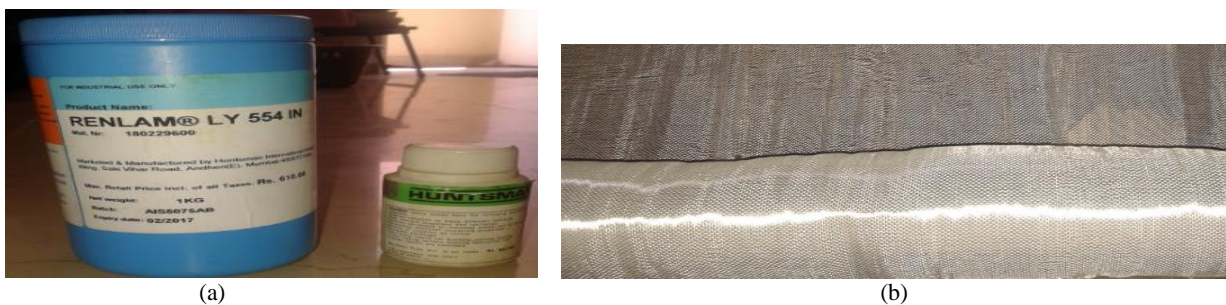
Fig 1: Resin Selection For Composites (a) LY 554 IN Epoxy and HY 951 Hardener (b) E-Glass Fiber Rolling Sheet
