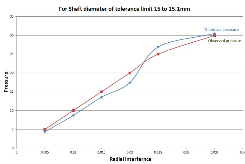
Fig. 5 Graph between pressure and radial interference for shaft diameter of tolerance limit 15 to 15.1 mm
