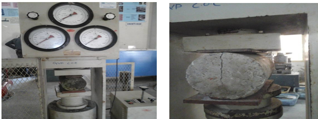
Fig 2: shows the split tensile set up for cylindrical specimen
