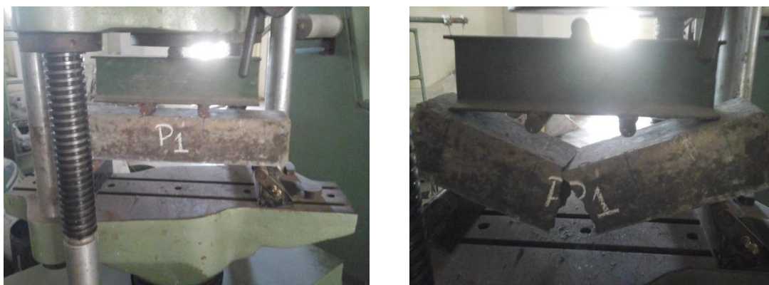
Fig 3: shows the flexural strength set up for beam specimen
