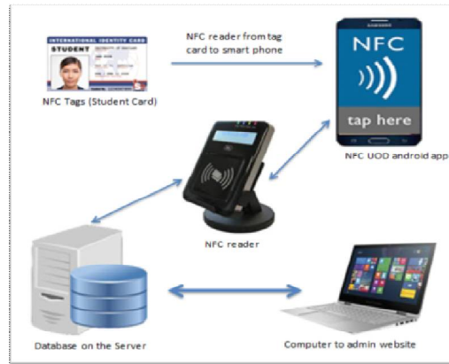
Figure 1: structure of NFC system used for students card
