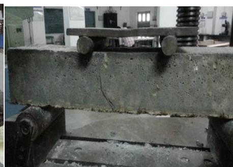
(c) flexural strength test
