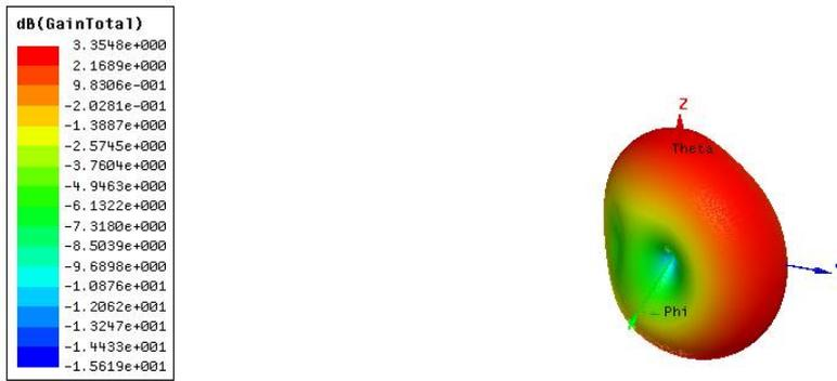
Figure 8: 3D Radiation Pattern at 13 GHz
