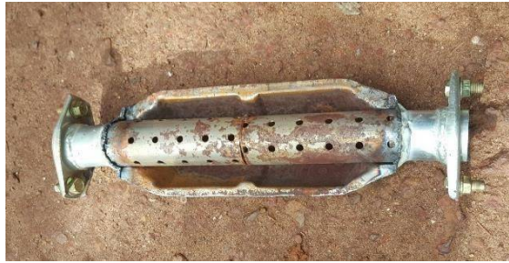
Fig. 1 :Cut section of catalytic converter
