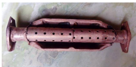
Fig.2.6 :Nano copper coated catalytic converter
