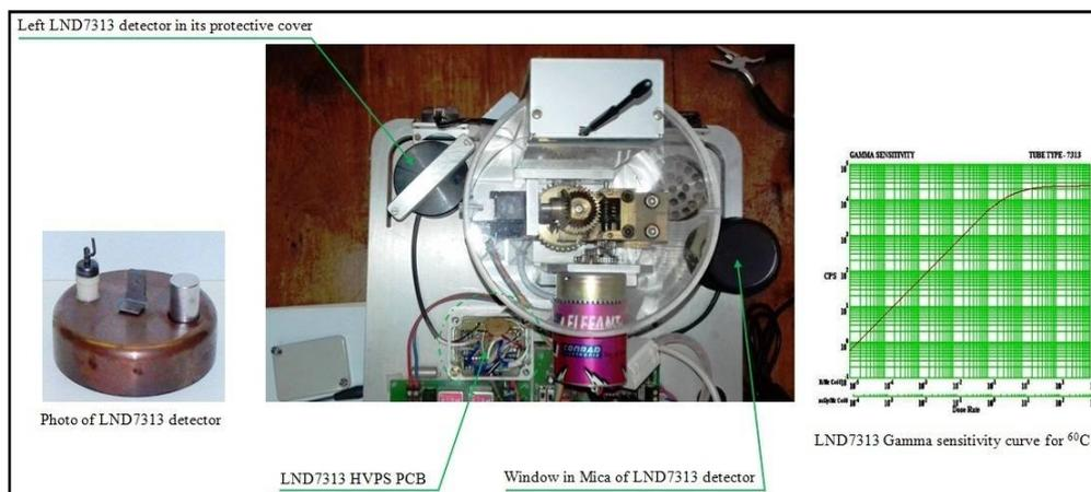
**Figure 3:** Photos of LND7313 detectors with their HVPS board and its gamma sensitivity curve related to <sup>60</sup>Co
