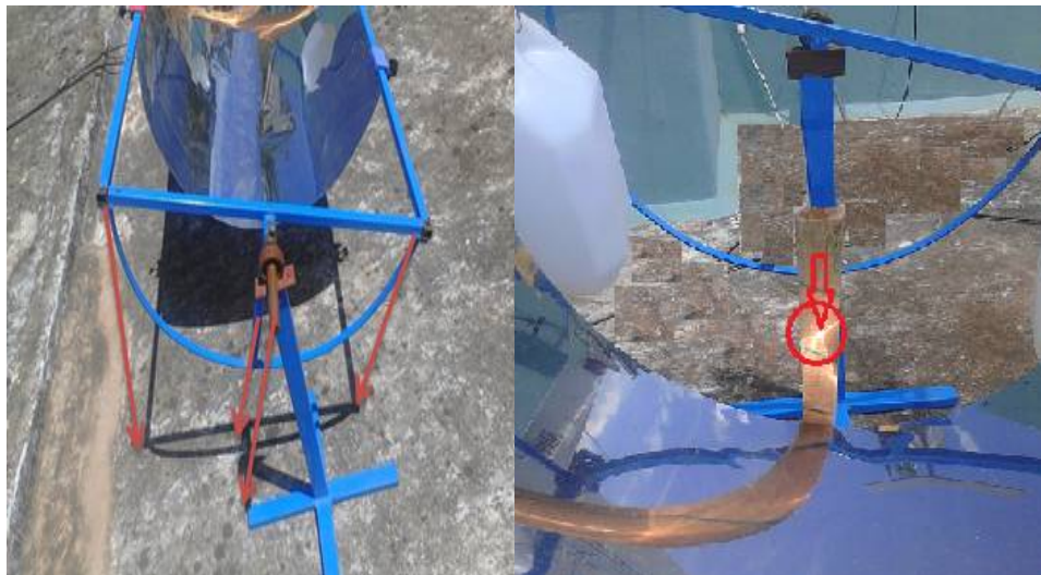
Fig. 9 Single axis tracking system focal point for both 1m and 2m parabolic system
