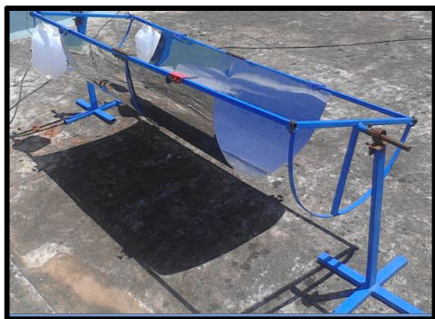
Fig. 5 Photograph of 2m Parabolic Trough with the Tracking System Fig. 6 Photograph of 1m Parabolic Trough with the Tracking System
