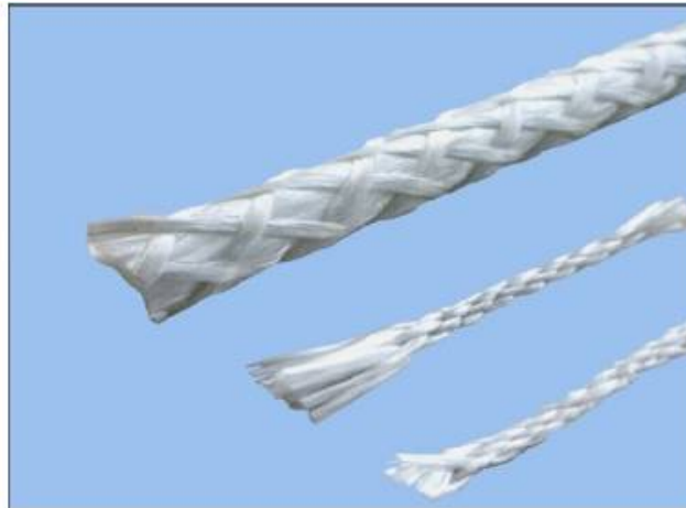
Figure2: Glass fiber in string form
