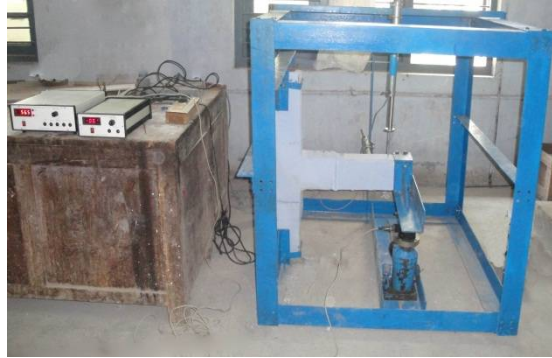
Fig. 4. Test setup with beam column joint
