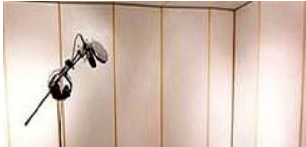
Figure 10: Record the SPL sensitivity by Condenser Microphone when the experiment room provided with Gypsum Board over it
