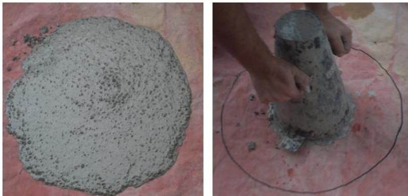
Fig (2) Slump flow test
