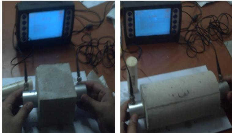
Fig (3) ultrasonic pulse velocity measurement for concrete cubes and cylinders
