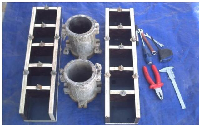
Fig 1: Details of Wooden Cubic Forms and Cylinders
