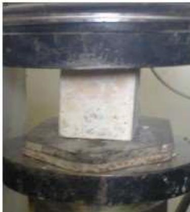
(Fig. 4a) Compressive strength test
