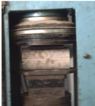
(Fig. 4b) Splitting tensile strength test
