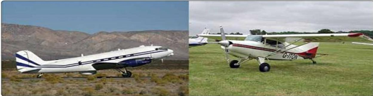
*Tail wheel configuration landing gear on a DC-3 (left) and a STOL Maule MX-7-235 Super Rocket.*
