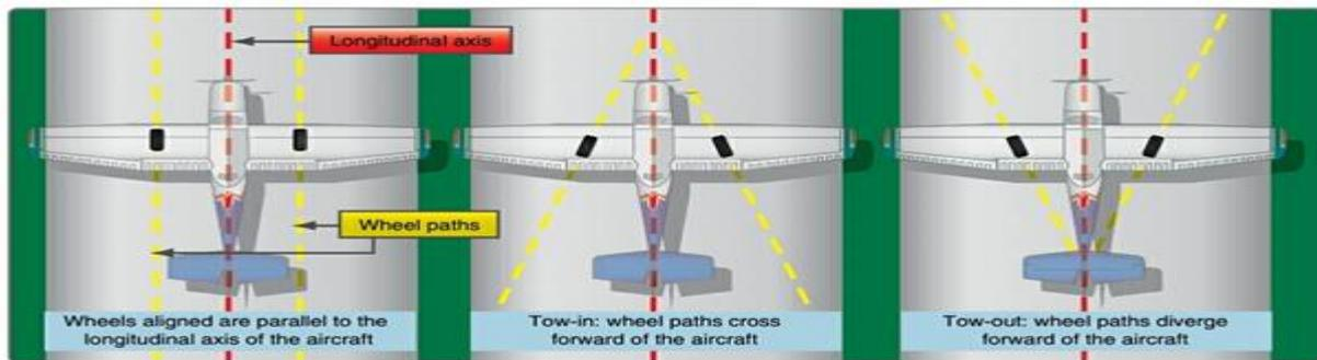
Wheel alignment on an aircraft.
