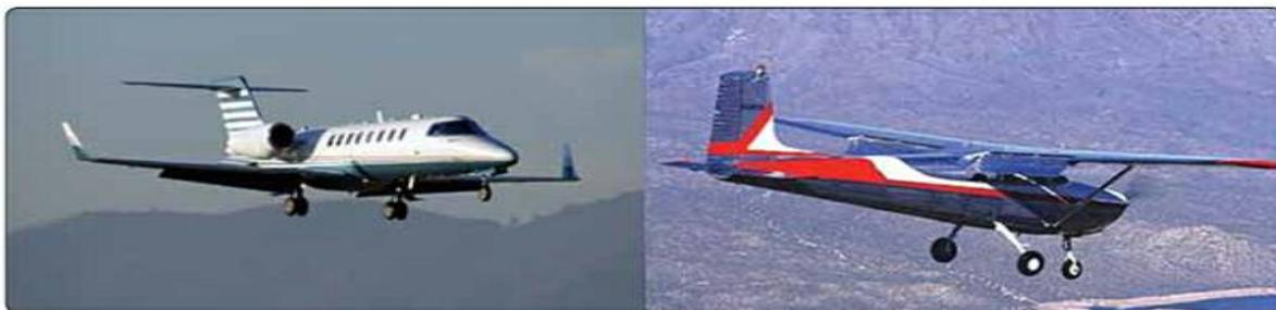
Tricycle-type landing gear with dual main wheels on a Learjet (left) and a Cessna 172, also with tricycle gear (right).
