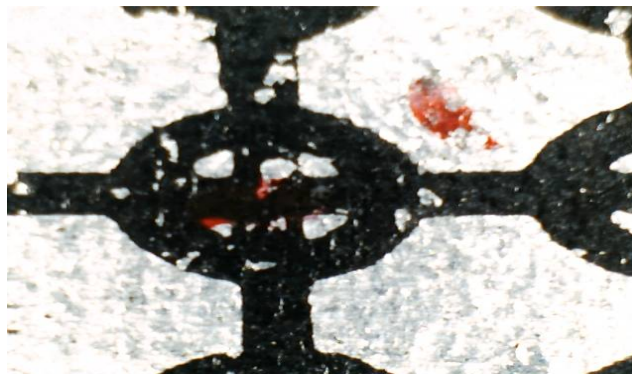
Figure 2.10: Grid formation after cupping taken using microscope
