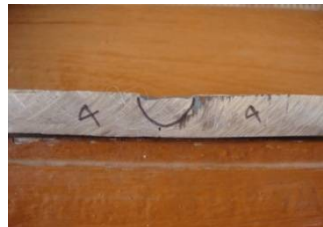
Fig 6.4 View of Test Plate -4 Peak Current-160, Basecurrent-18 , TOR AN -45
