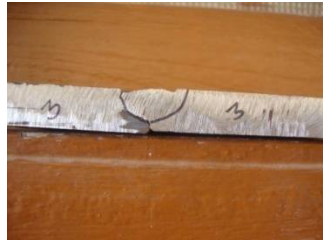
Fig 6.3 View of Test Plate -3 Peak Current-14 , Basecurrent-22 , TOR AN -60
