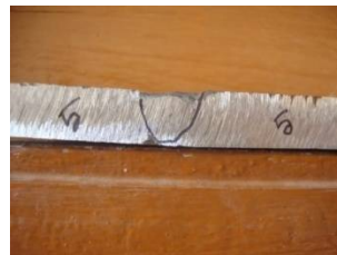
Fig 6.5 View of Test Plate -5 Peak Current-160, Basecurrent-20 , TOR AN -60
