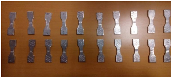
Fig 5 Specimen before Tensile testing(ASTM E04)
