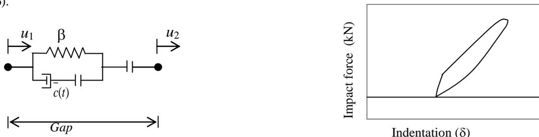
a) Structural configuration of gap element
