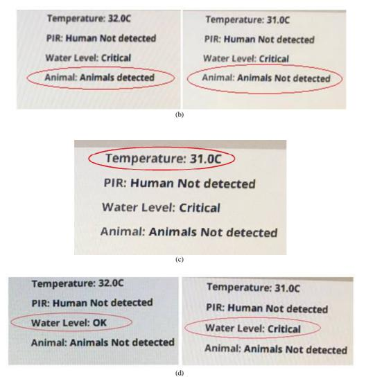
Fig 3. Website display of results against the corresponding labels (a) Reading of the PIR Sensor when the human presence is detected and not detected. (b)Reading of the Pressure Sensor when the animal presence is felt and not felt. (c) Reading of the Temperature Sensor in degree Celsius (d) Reading of the Float Sensor when the water level is satisfactory and critical.
