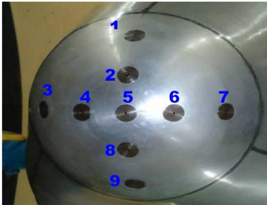
Fig 1: Pressure ports on nose cap
