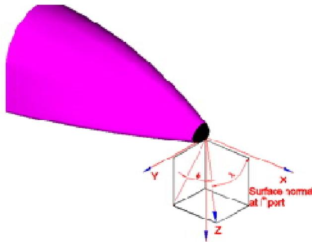
Fig 2: Definition of cone angle and clock angle
