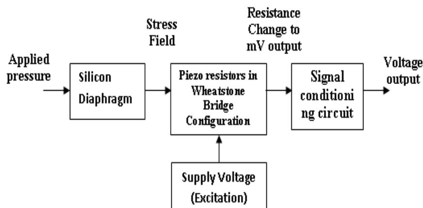
Fig 3: Block diagram of MEMS pressure transducer
