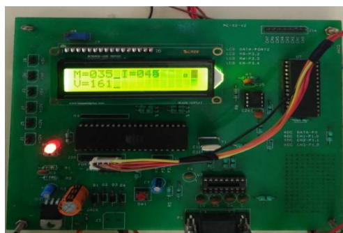
Figure 5: Displaying amount, current and voltage consumed
