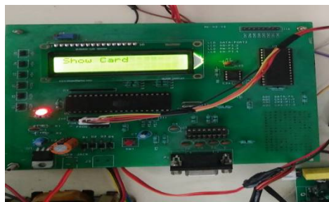
Figure 3: Displaying show card to place the card in RFID reader
