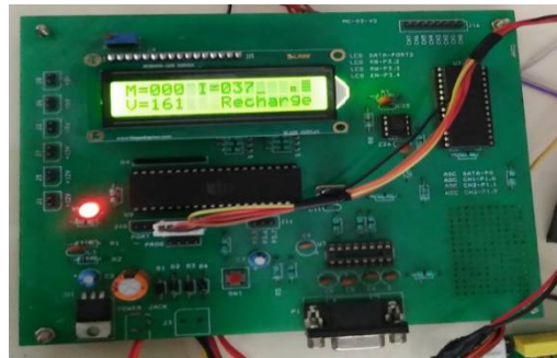
Figure 6: Amount is zero and indicating to recharge
