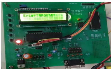
Figure 4: Displaying Enter amount to select the amount in keypad
