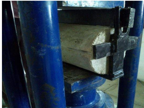
Fig. 5: Testing of cylinders for Split tensile strength
