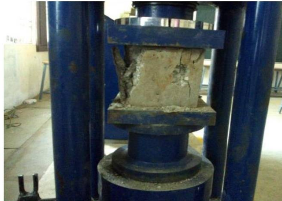
Fig. 4: Testing of cubes for Compressive strength
