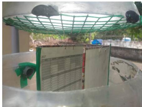
Fig. 4. Baffles within the Primary Settling tank
