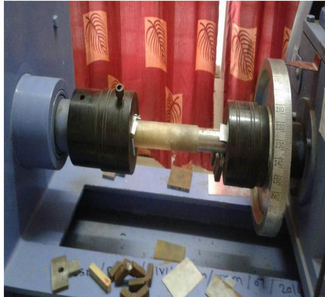
Fig-3. Experimental set up for torque testing
