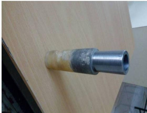
**Fig-1.**Composite shaft before machining
