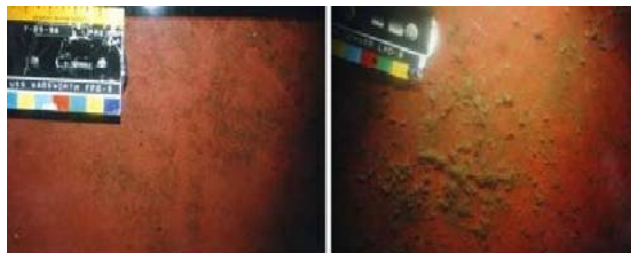
Fig 2. 7 Reference pictures of “thin slime” (left) and “thick slime” (right)
