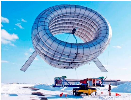
Fig 2.2 Buoyant Airborne Turbine
