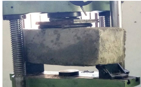
FIG 1.5. FLEXURAL TEST AFTER RETROFITTING
