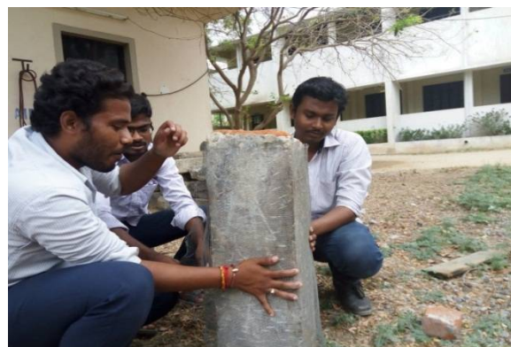
FIG 1.3.BEAM WRAPPED WITH MESH
