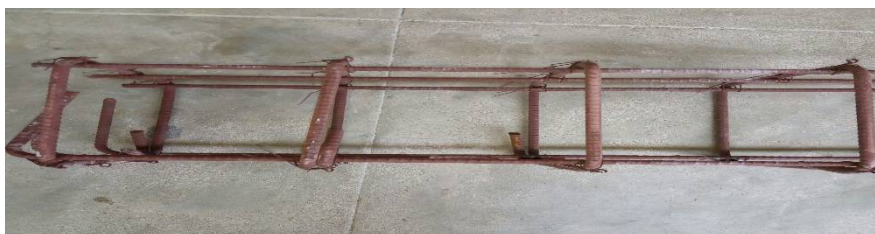
FIG 1.1 REINFORCEMENT DETAILS OF THE BEAM
