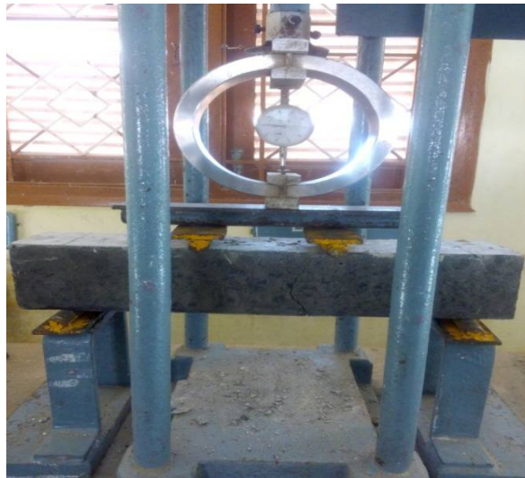
Fig 4.2 Test Set Up for Flexural Strength
