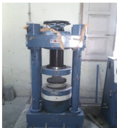
Fig 4.1 Test Set up for Compressive Strength Test
