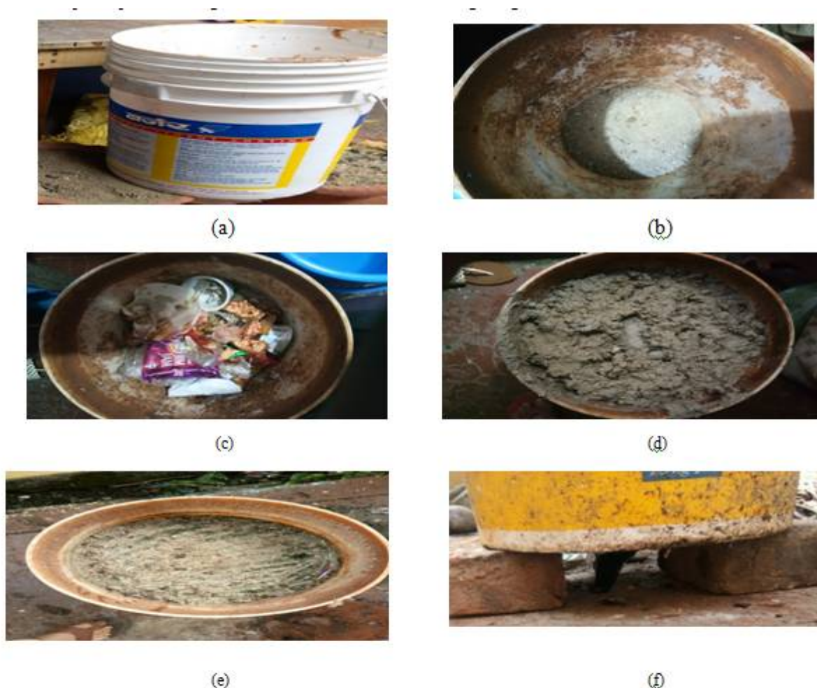
Figure 6: (a) 25 liter container for landfill model (b) \frac{1}{3}^{\text{rd}} of container filled with flyash – 16% flyash mixture (c) Household waste on the layer of Flyash- 16% bentonite mixture. (d) Compacted layer of Flyash – 16% bentonite mixture on household waste, (e) Landfill liner after 8 days of rain. (f) Leachate collected after 13 days.
