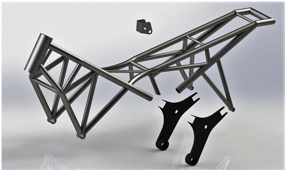
Fig.1: Exploded View of Trellis Frame and Components
