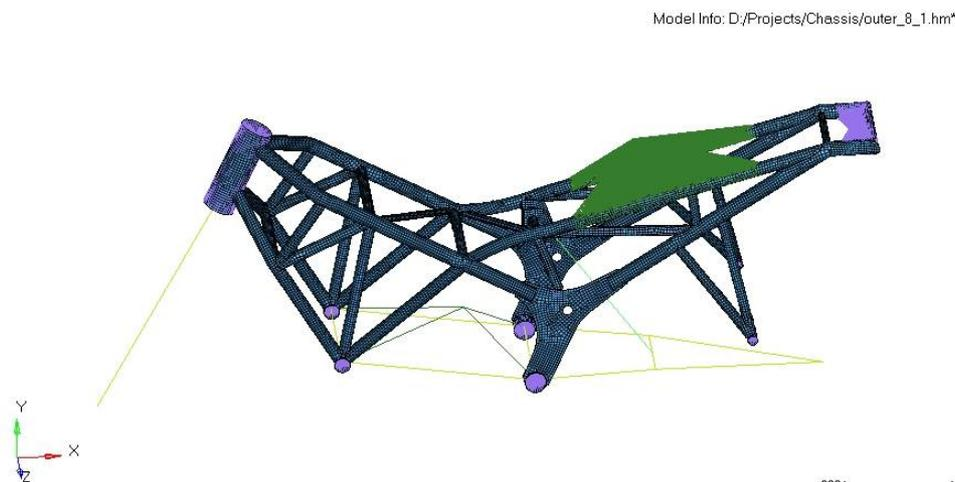
Fig.3: Mesh Model of Frame
