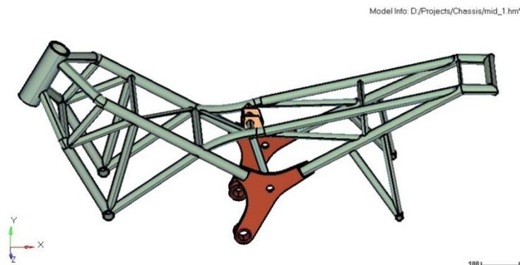
Fig.2: Assembled Model of Trellis Frame
