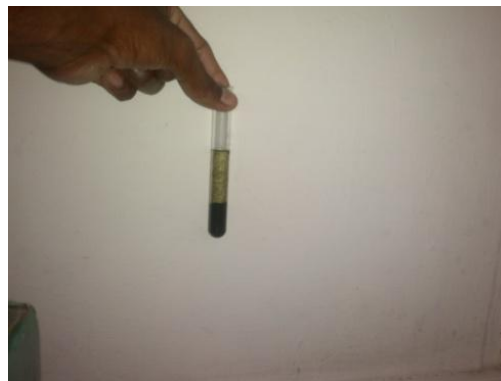
Fig. 5 CNTs in a test tube after centrifugation
