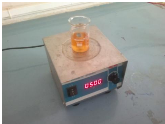
Fig. 3 Magnetic stirring of PdCl 2 and HCl
