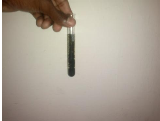
Fig. 4 CNTs in a test tube before centrifugation
